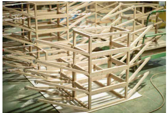
Group of assembled red oak modules at the workshop
